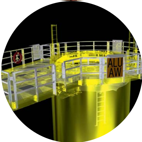
Aluminium platform constructions made of sheet and extrusions for offshore wind turbine foundations, built by Aluwind A/S.
