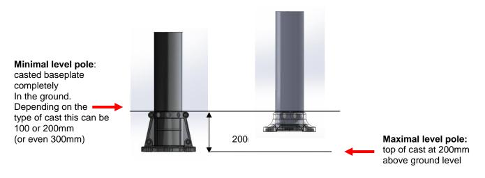
Note: the red arrow is ground level in both extremes; the 200mm comes from STRMTG: GT3-DTW-Obstacles Fixes V2. The pole needs to break below 200mm above ground level with maximal 570 daNm.
