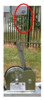
**Note:** Check all connections are secured and make sure that the cable is secured. Ensure the cable is tightened prior to loosening captive bolts. This to check if all is secured! Then move on to the "lowering and raising of the hinged column", *Section 7*.
