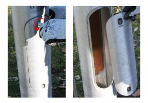
2. Mount the winch bracket including clamp onto the parallel part of the column as shown. Tighten the two M16 bolts. As a visual guide, mount the winch bracket in line with the center of the wedge.
