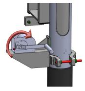
Once the work is completed, Steps 1 to 9 should be carried out in reverse order. Make sure that the 4x (3x for D145mm column) internal captive M12 bolts are torqued to 50Nm.
