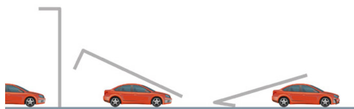
NE mast: Non energy absorbing
