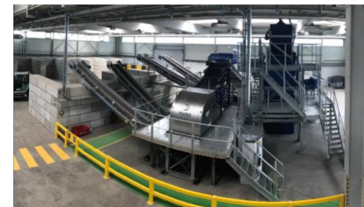
LIBS pilot in operation in St Peter sorting plant
