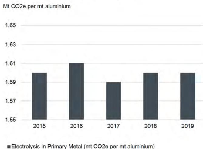
Greenhouse gas (GHG) emissions from the electrolysis process from Hydro's smelters, excluding Neuss in Germany. Albras is excluded from the 2019 average due to extraordinary emissions during start-up of curtailed capacity. The emission intensity at Albras was 1.89 in 2019.
