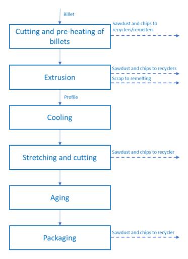
Figure 1: Scheme of the manufacturing process occurring at Hydro Extrusion Nenzing GmbH extrusion site.
